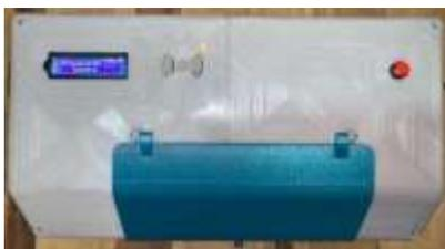
Figure 1: Polarimeter prototype.
