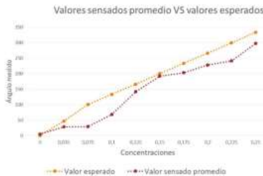
Figure 2: Contrast of average sensed values with analytical calculated values.
